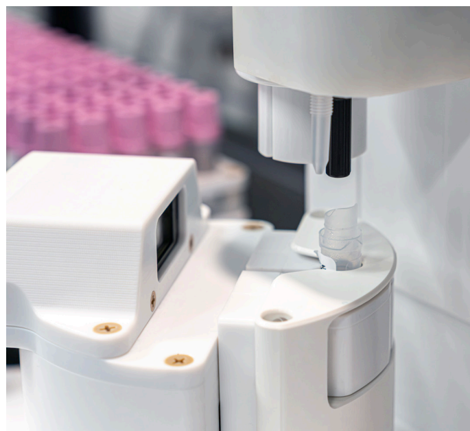
Figure 3. LinkGauge detects presence and volume of microsamples automatically.
