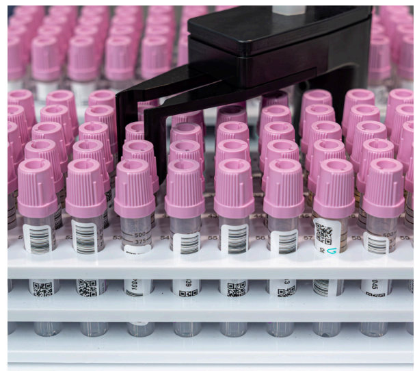
Figure 1. Capillary collection tubes on the TRAXStation Clinical .
